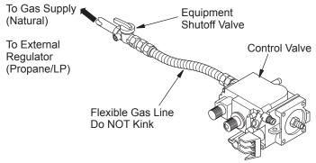
Figure 32 - Connecting Flexible Gas Line to Millivolt Valve
